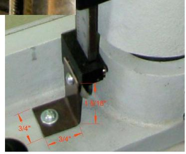
Finally, cut another small piece of angle as per the dimensions to the gauge bracket the hole for the bottom the cutterhead all the and note if the bracket point you may have to of the top mounting slightly bend the angle body so that the does not move through the range of cutterhead. Then drill bottom machine screw
